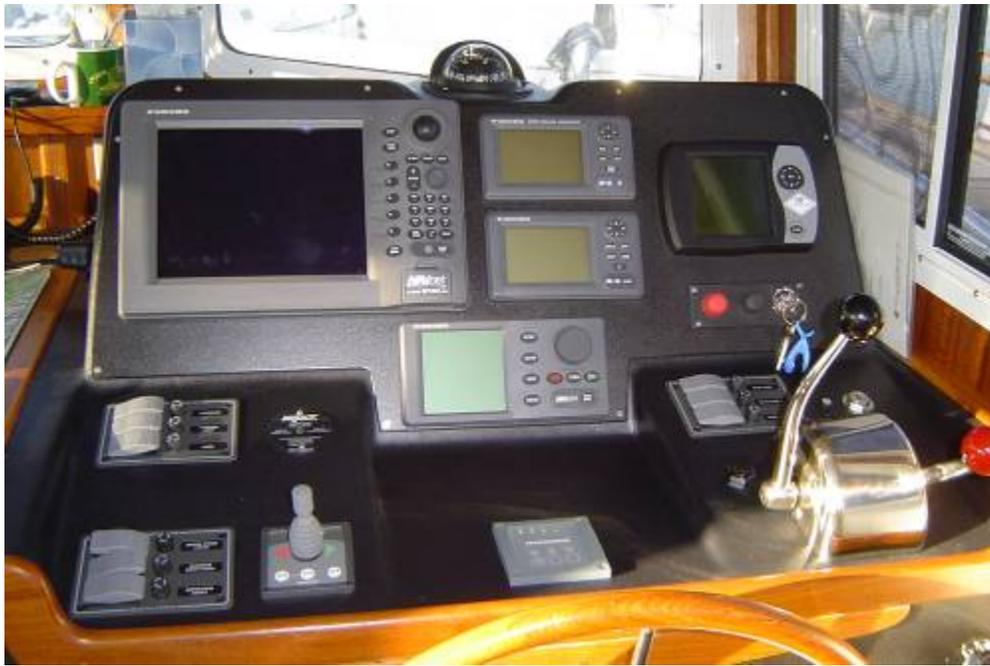
Anacortes Marine Electronics installed Furuno radar, chart plotter, auto pilot, depth finder, GPS and two Icon radios.
