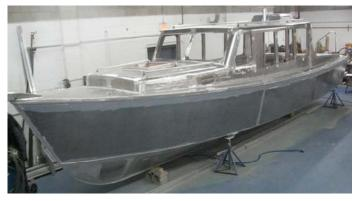
The welded aluminum construction makes it very strong and safe. Being aluminum it does not need to be painted, however, a colored hull with bottom paint may be preferred. Designed with an 8-foot beam, it is legally trailerable anywhere in the US and weighing approximately 7,000 pounds it can be pulled with a modest tow vehicle.
