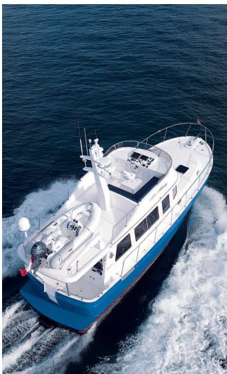
according to Bracewell, concentrates a good share of the yacht's displacement low and near the centerline. Moreover, a noticeable bulge just aft of amidship creates a depression in the mechanical space that allows the single diesel engine to be positioned below what the nominal bottom contours otherwise would permit.
