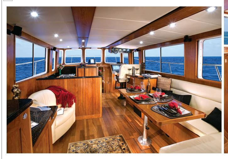
Overhead beams reinforce the top of the deckhouse, freeing the interior from the intrusion of structural posts and bulkheads.
