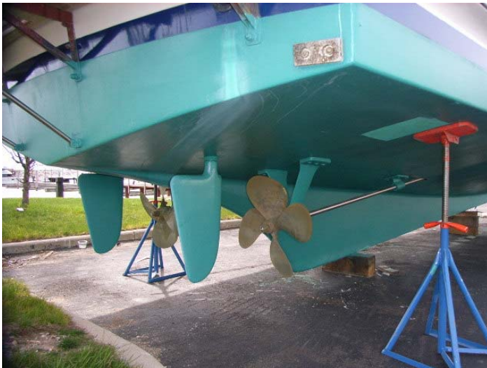
Hull design with twin engines, unprotected props and shafts
